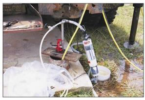
Water-quality sampling—Samples were collected from three wells to determine water quality. A pump is set into the well to collect the samples. Water-quality properties are monitored during the process of purging the well prior to sampling. Photo by Lester J. Williams, USGS.
