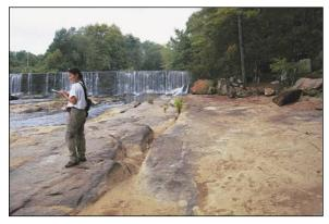
Geologic mapping—Rock types, joints, fractures, and other water-bearing features are mapped by walking along roads, riverbeds, power lines and other access points. The above photo shows a prominent set of joints aligned parallel to the streambed of the Yellow River near Milstead, Georgia. Photo by Lester J. Williams, USGS.
