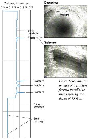
A caliper log is the simplest log to interpret. Peaks show where the borehole is enlarged and indicate sections of the borehole where a fracture opening may be present.
