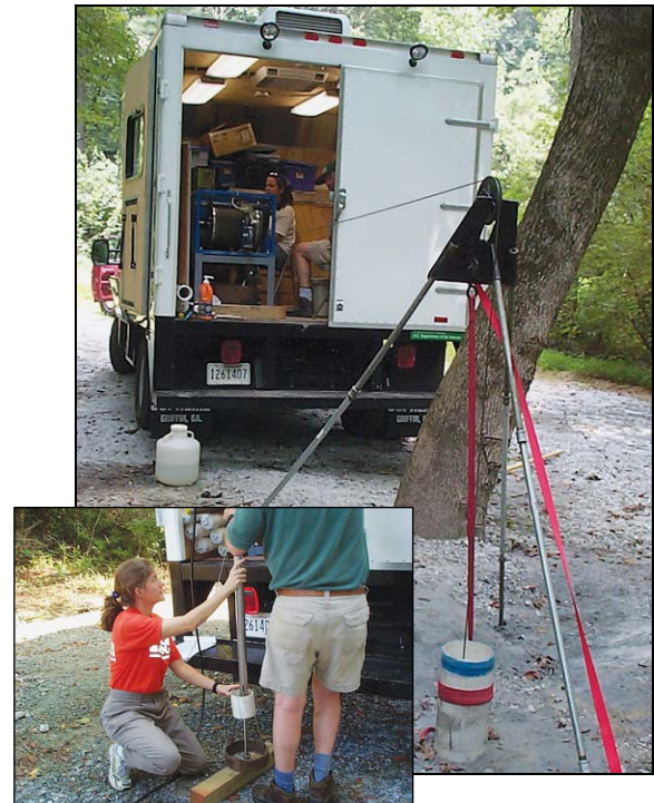
Figure 1. Logging a 6-inch-diameter crystalline-bedrock well in Lawrenceville, Georgia. Inset shows a three-arm caliper tool being calibrated with a steel ring. Photographs by Lester J. Williams, USGS.
