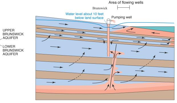
Floridan aquifer, causing direct connection between seawater and fresh ground water. Regional ground-water pumping, but most importantly,
