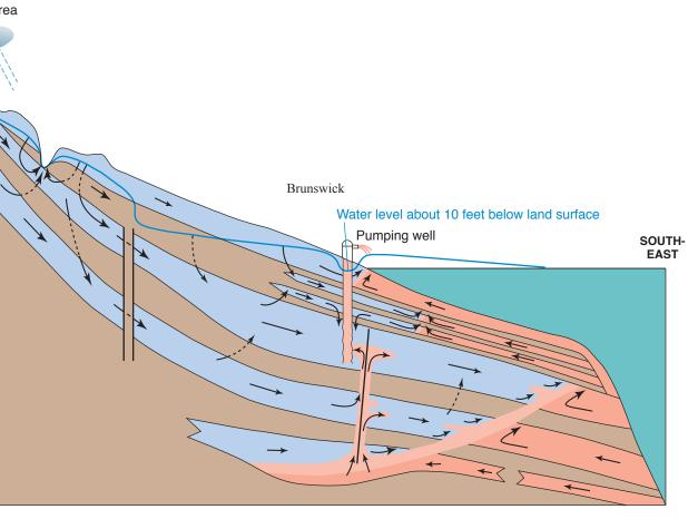
Freshwater in the aquifer system along the coast also has an interface with saltwater at depth. Saltwater occurs naturally in aquifer-system sediments below the freshwater zone, extending landward from the freshwater-saltwater interface offshore, and underlying freshwater in the
