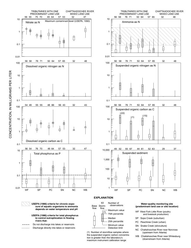
Figure 2. Nutrient and suspended-sediment concentrations during baseflow and stormflow conditions in the upper Chattahoochee River basin, 1993–98.
